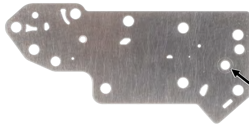
Lock-up solenoid pulse damper
