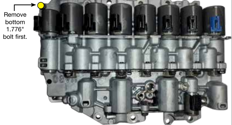
UA80E Solenoid Valve Body Front Side
