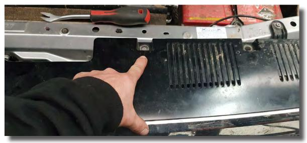
1.3. Ensure all bolts are removed, they are located not only on the radiator support bar but also on each side headlight.
