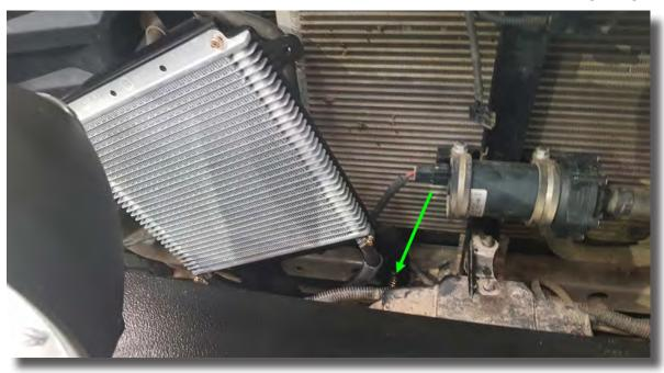
1.10. Slide the cooler in to position carefully and attached supplied M8 Bolt and Nut (M6 also supplied if necessary) through the vacant hole in the lower support panel that aligns with the lower left bracket mount.
