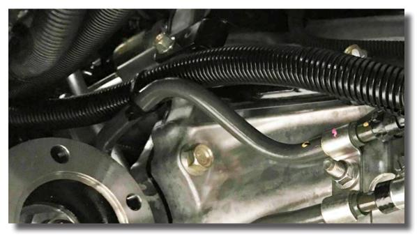
Run the cooler line down beside transmission and existing cooler lines and connect to centre outlet on OEM heat exchanger. Secure with supplied screw clamp.
