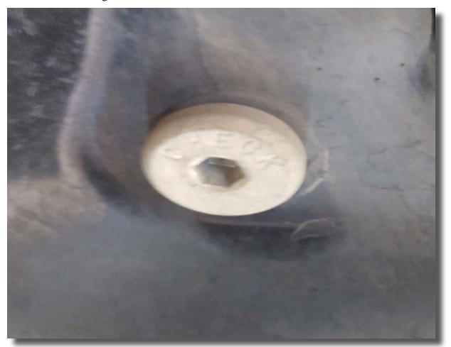
With the engine running, remove using a 5mm Allen key. DO NOT remove the 14mm bolt located at the rear of the transmission pan as this is the drain plug.
