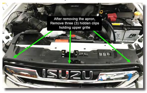
5. Remove the (1) phillips head screw in the center of the grill located just under the Isuzu front badge.
