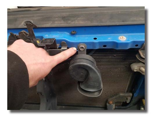
Unbolt and remove the bracket holding the air conditioning line. Refer the 5. photo below.
