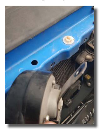
Bolt the supplied cooler bracket's top bolt hole and the horn (flipped to face the reverse direction) to the original horn mounting hole.
