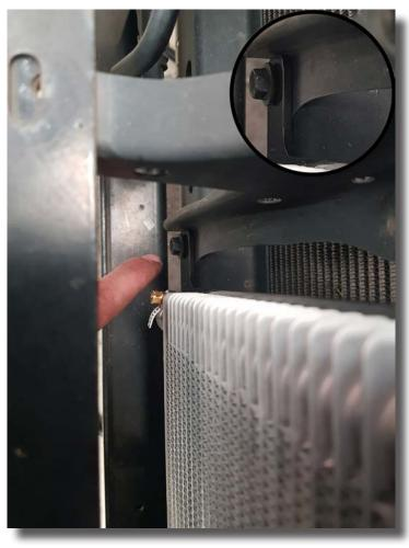
Install the plastic clip in the square hole of the angle bracket supplied with 13. your cooler bracket. Bolt (use factory bolt removed earlier) the angle bracket and cooler bracket together to the vehicle via the bottom right hand bolt hole in the cooler bracket. Clip in air conditioning line. See photo below.
