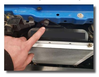
Note: in the above photo the horn is hidden behind the supplied cooler bracket.
