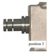
**Position 3** ATF fully bypasses the cooler (i.e., No cooler flow!) THIS IS A TEMPORARY QUICK WARMUP SETTING to bring trans to required temp to RESET THE COMPUTER. Once relearn is initiated, set the adjuster to Position 1 or 2
