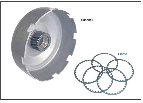
**NOTE:** Sonnax shim **36414-01K** is .044" thick. Its tooth cut will not allow the shim to be easily pushed over the sun gear. The sun gear will be a press fit inside the shim, which requires the gear to be pushed/driven through the shim before installation.
