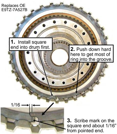
**4.** Then grind the square end to the mark and reinstall ring.
