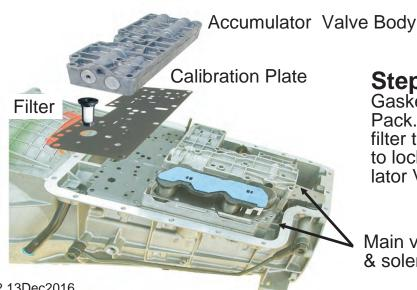
**Step 2.** First install the Separator Plate, Gaskets, Main Valve Body & the Solenoid Pack. Then install Calibration plate. Insert filter thru both plates and rotate it 1/4 turn to lock it in place. Last install the Accumulator Valve Body. It's OK without a gasket.
