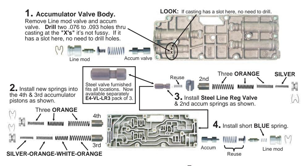
LOOK: If casting has hole EX, no drilling needed.
