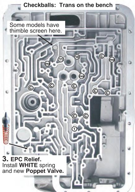
If plate has hole 89, install all 11 balls. If plate has hole 90, don't use ball 10 & 11. If plate has hole 2T, don't use ball 1, 10 & 11. When used: Ball 10 must be 5/16" steel, all others 5/16" plastic.
