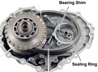
**Helpful Tip:** After releasing tension on belt, lift the secondary pulley & puller straight up out of bearing pocket and slide it into the belt area of the primary pulley to overlap the pulleys. The belt will now fall outside the secondary pulley. Tilt secondary pulley assembly toward the primary pulley to lift secondary out of the belt and off the rear case cover onto the bench. Remove the puller & Strap Clamp.
