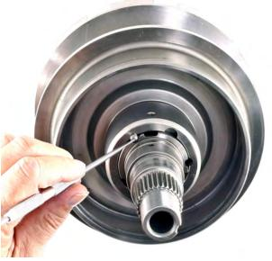
It may be necessary to push each ball into the groove with some light pressure. Do not use a hammer! A little pressure and wiggling of the sheave and they will go right in.
