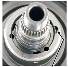
Line up Hump on snap-ring to half-moon groove in sheave.
