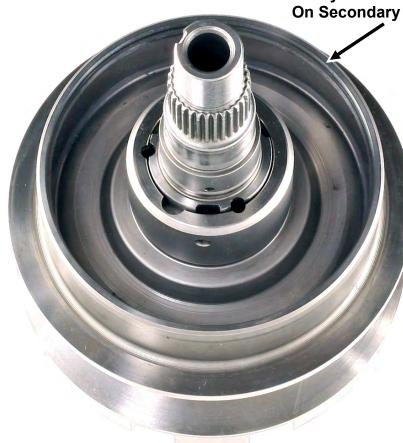
Lubricate the Secondary Shaft & Ball grooves with approved CVT fluid. Align the Pulley Sheave carefully until it will slide down the shaft.
