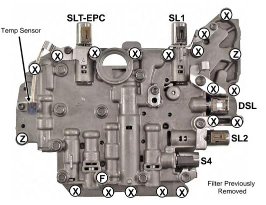
SL1, SL2 & EPC 5-5.5 Ohms between pins S4 & DSL 11-15 Ohms between pins From Either Pin to Body of Solenoid must be open!
