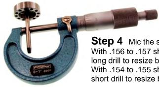
Step 4 Mic the shaft. With .156 to .157 shaft use long drill to resize bushings. With .154 to .155 shaft use short drill to resize bushings.
