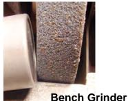
**Step 2** On the angle shown, using the SIDE of the grinding wheel, grind off the crimped end.
