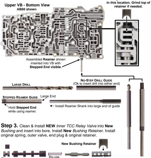
New Inner TCC Relay Valve & Bushing
