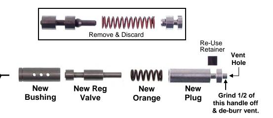
**Heads Up!** We have had reports that on SOME models the handle of the new plug MAY touch the pan or case. Therefore, on A760, A761 & A960 models grind the handle of the plug down about half way & de-burr vent hole before installing. Make sure the vent hole is open.
