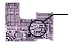
Fits Valve bodies with 2 or 3 SMALL balls located in this area and has F6 or F8 code on main VB.
