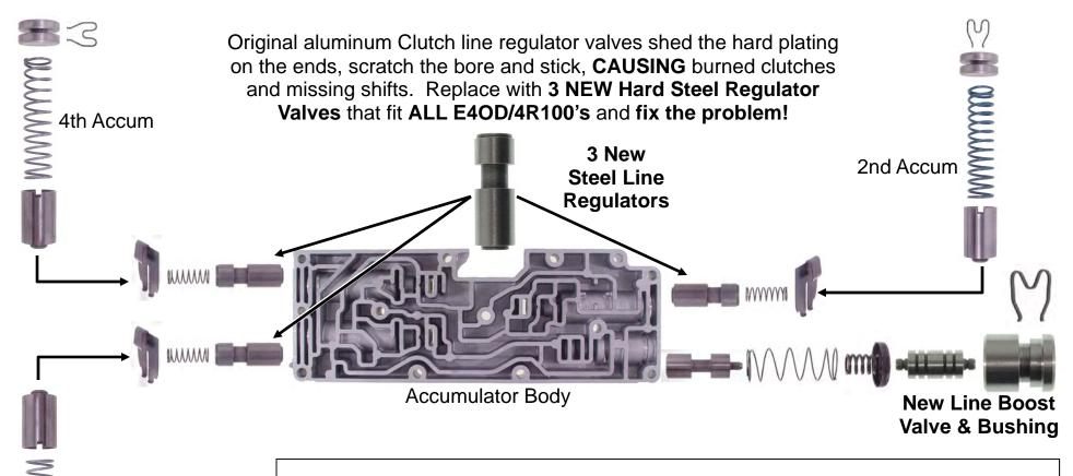
**NEW STEEL: Line Boost Valve & Bushing** replaces worn original equipment .372 diameter aluminum valve & bushing that can cause soft shifts.
