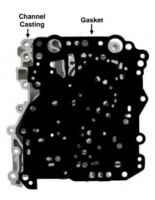
**2.** Enlarge separator plate hole with .110 drill provided before final assembly of channel casting.
