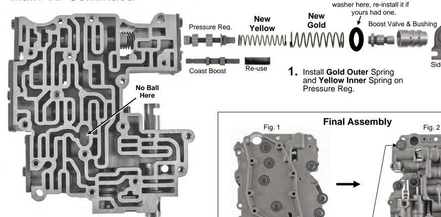
Lay completed Channel onto Completed VB (Fig. 1) and Install 7 short bolts but do not tighten. Flip VB over and install 2 Large bolts as shown in fig 2. Tighten large bolts first and then 3 small channel plate bolts. Flip VB back over and tighten 7 bolts as shown in fig 1. Install filter and tighten filter bolts, then tighten side plate bolts last. Tighten small bolts with a spin-tight or nut-driver. 2 Large bolts and VB to Case bolts Snug with a short wrench.
