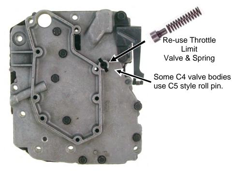
**C4 Models:** Install Throttle limit valve and spring before installing filter!
