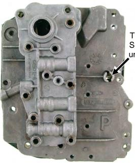
Throttle Limit Spring visible under roll pin.
