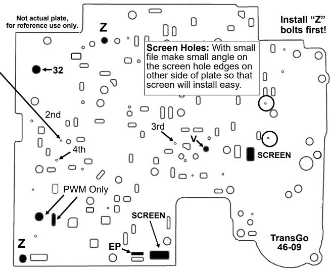
2009: Must have PWM solenoid and holes EP, V. Has NO 3-2 Solenoid or hole 32.
