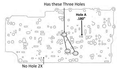
Type 2 Plate, Version 1 Used on Type 2 VB's thru 2013 Has the 3 circled holes & .180" feed hole A. No Hole 2X Install Check Balls 1-7 It is a good idea to update this Type 2 Version 1 plate to a Version 2 during repairs and add the #8 check ball. Plates are cheap and come with bonded gaskets.
