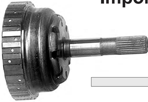
Drill cup plug in underdrive hub .086 to .096 to increase lube flow to the planets.
