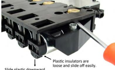
Slide plastic downward to re-install insulators.
