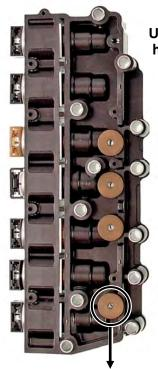
Use a small amount of assembly gel to hold the parts in place before putting module side onto solenoid side.
