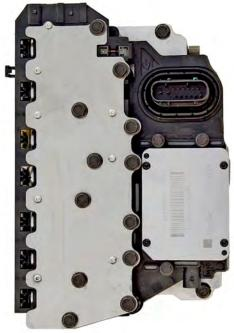
All Solenoids = 4.0-5.0 Ohms Except On/Off = 16-20 Ohms N.C. PCS-4,5 & TCC Normally Low (output) PCS-2,3 & EPC Normally High (output)
