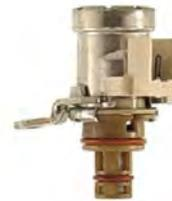
TCC Control Solenoid often fails causing “Chugs” or “Kills” engine at stop. Replace it.
