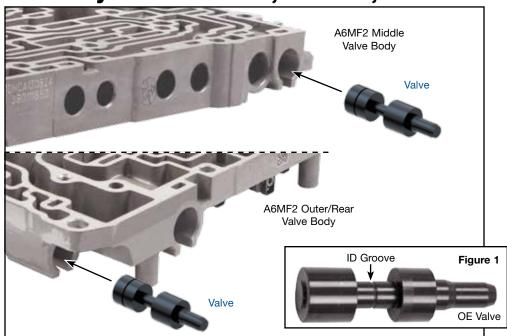
**NOTE:** If OE valve has ID groove between the two spools (**Figure 1**), adjustable end plug MUST be measured and adjusted. See step three below for details.
