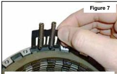
Orient the spring retainer as shown, with the free part of the spring facing out and the retainer towards the O.D. of the housing.
