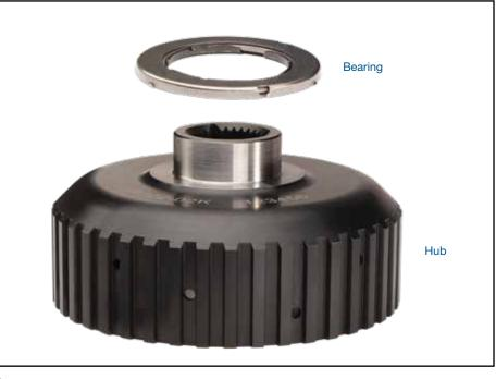
**WARNING:** Compared to OE or other replacement forward clutch hubs, this hub and bearing combination has an additional .025" thickness designed-in to reduce endplay and provide further endplay adjustment options.
