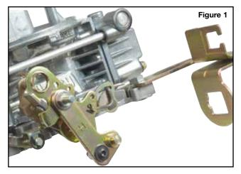
5. **Checks and Verification:** With the throttle in the idle position, mark the cable where it enters the cable housing. Rotate throttle arm and hold in the wide-open throttle position with the cable pulled out of the cable housing. Measure distance between mark on cable and cable housing. Distance should be 1.48" (1-31/64") for the GM 4L60 and Ford AOD (**Figures 2 & 3**, page 2).
