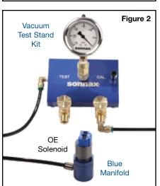
NOTE: Sonnax test manifold kit can prove or disprove internal mechanical sealing ability only; it does not test the integrity of the electrical coil and contacts. While internal mechanical sealing problems are the leading cause of failure for this family of solenoids, electrical testing should also be carried out to confirm comprehensive solenoid operation.
