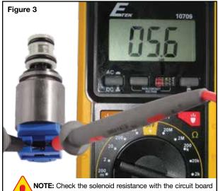
NOTE: Check the solenoid resistance with the circuit board removed. For orange, blue or yellow capped solenoids, resistance value should be 5-6 ohms at 68° F.
