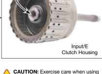
a puller to remove bushing, as it is possible to inadvertently cause grooving of the bore with the puller arms. These grooves can prevent the mating
