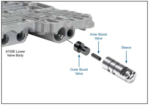
**NOTE:** Before disassembly, note position of retainer on OE sleeve. Retainer must be returned to the corresponding step on Sonnax sleeve during installation.
