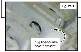
**NOTE:** If a line-to-lube orifice has been drilled into the pump casting wall, it must be plugged (**Figure 1**).
