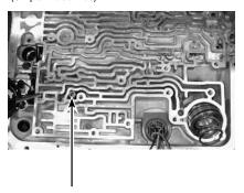
The check valve Installs on top of the OE 3rd accumulator capsule.
