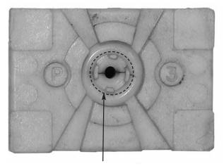
Inspect the TCC solenoid seat for cracks.
