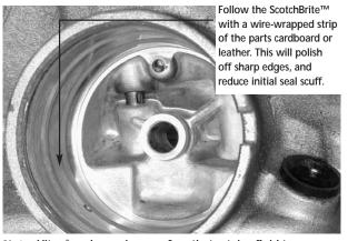
Note: Viton\* seals require a surface that retains fluid to ensure long life.
