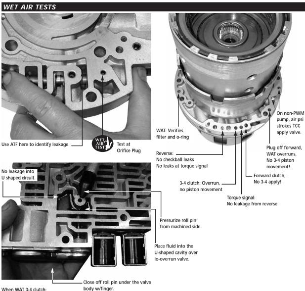
When WAT 3-4 clutch: No oil loss at checkball, or base of shaft.
