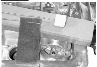
Use a fine grit stone to remove high spots on case and valve body. Scuff the accumulator(s) and servo bore with Red ScotchBrite™. A stiff wire or rod wrapped with material can be spun in a drill.
