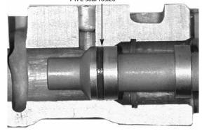
PTFE seal supplied must be stretched to install into valve groove. Resize with finger pressure, pre-lube, then resize by inverting into bore.
