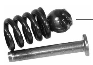
Remove the relief rivet and clean ball and seat. With severe contamination, reform the seat by tapping ball into it.
