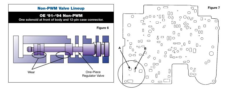
NOTE: Since the castings for PWM and non-PWM valve bodies are identical, this kit can be used when updating a non-PWM valve body for use in a PWM unit or retrofitting a PWM valve body for use in a non-PWM unit. The separator plate must also be changed when this is done (Figure 7).
