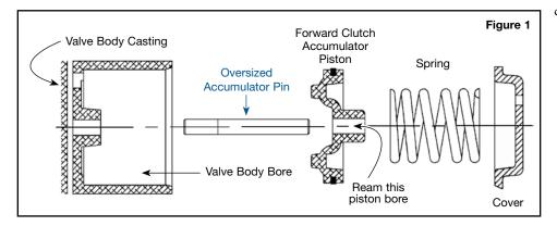
c. Reinstall OE Forward clutch accumulator piston with new seal (*not supplied*), spring, cover and retaining bolts.
