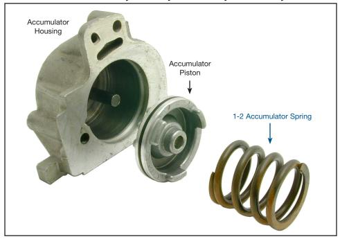
Sonnax performance-rated 1-2 accumulator spring 77704S provides firmer shifts for the enthusiast that appreciates quick, positive shift feel in GM 4L60-series units. The spring design provides performance shift feel, but does not reduce accumulator piston travel. This allows for a firmer - but still cushioned - shift that minimizes shock to the band and shafts.
