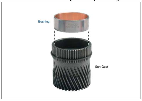
Install bushing using arbor press.
