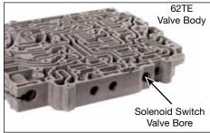
NOTE: Large spool of OE switch valve must be .420" dia. (main photo). If spool measures .420", continue installation. If spool measures .453", STOP! This Sonnax kit cannot be used. Instead, install Sonnax oversized solenoid switch valve plug kit 92835-22K after reaming bore with Sonnax tool 92835-RM22.
