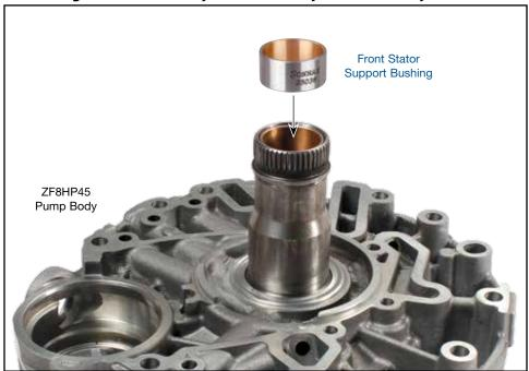
**CAUTION:** Use of an arbor press is required for correct installation. Do not use a hydraulic press or a bushing driver/hammer combination to install, as doing so will distort the bushing and cause fitment issues.
